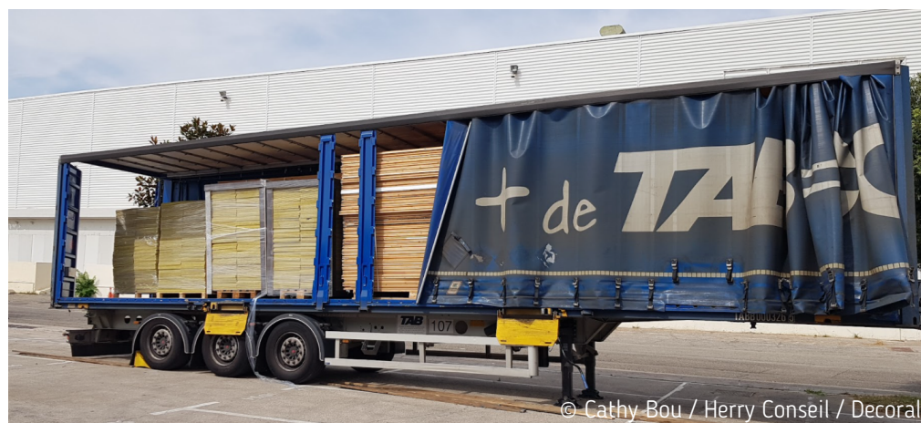
Transport module for piggyback transportation
